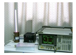
Fig. 1. Ionized plasma antenna prototype.
